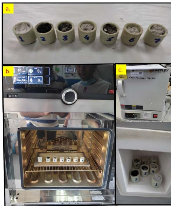
FIGURE 4. (a) Residue samples of seven different incinerated waste under test. (b) Sample heating in the oven for calculating moisture content of fly ash. (c) Sample heating in a muffle furnace for calculating loss on ignition of waste residue.
