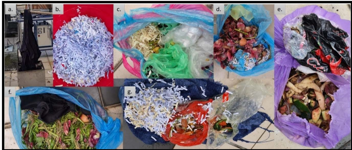
FIGURE 3. Variety of Municipal waste used for incineration test (a) Textile waste; (b) Paper waste; (c) Food waste; (d), (e), (f), (g) Mix waste.
