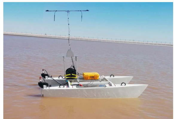
FIGURE 7. EDSON-J on a regular mission for water quality monitoring in a huge reservoir in Majes - Arequipa (latitude: -16,388 longitude: -72,195 ). This reservoir contains about 50\,000\,m^3 of fresh water from the Andes for rural irrigation in the city.
