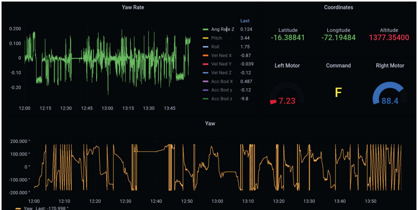
FIGURE 8. The graphical user interfaces for monitoring the navigation of the USV EDSON-J, the graphs belong to the tests carried out in the VR4 reservoir in Majes - Arequipa with a duration of 2 hours, the interface shows the register of all the data in time.
