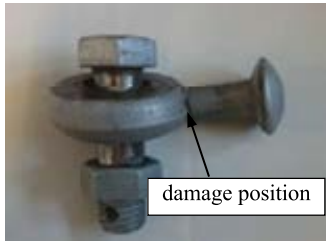
FIGURE 34. Fracture of ball head hanging ring Han et al.
