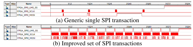
FIGURE 5. Comparison of a single 32-bit transaction via the generic SPI interface with the entire set of fourteen 32-bit transactions required for the retune procedure applying the proposed method. Both analyses are displayed on a common time scale.
