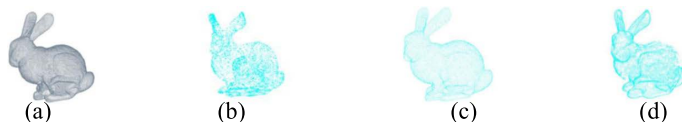
FIGURE 8. The simplification of rabbit. (a) original, (b) the proposed method, (c) grid method, (d) curvature method.
