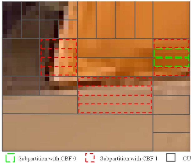
FIGURE 5. Example of CBF distribution of CU blocks encoded in the ISP mode (partyscene video, (QP=27, 1st frame), CUs at (224,392) to (264, 424)).
