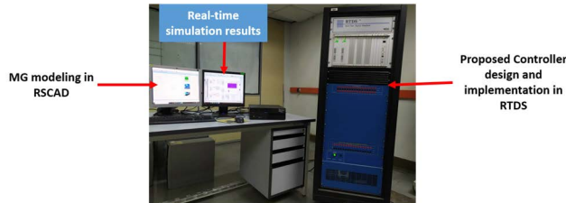
FIGURE 4. Proposed AC MG's PV VSI controller laboratory setup.
