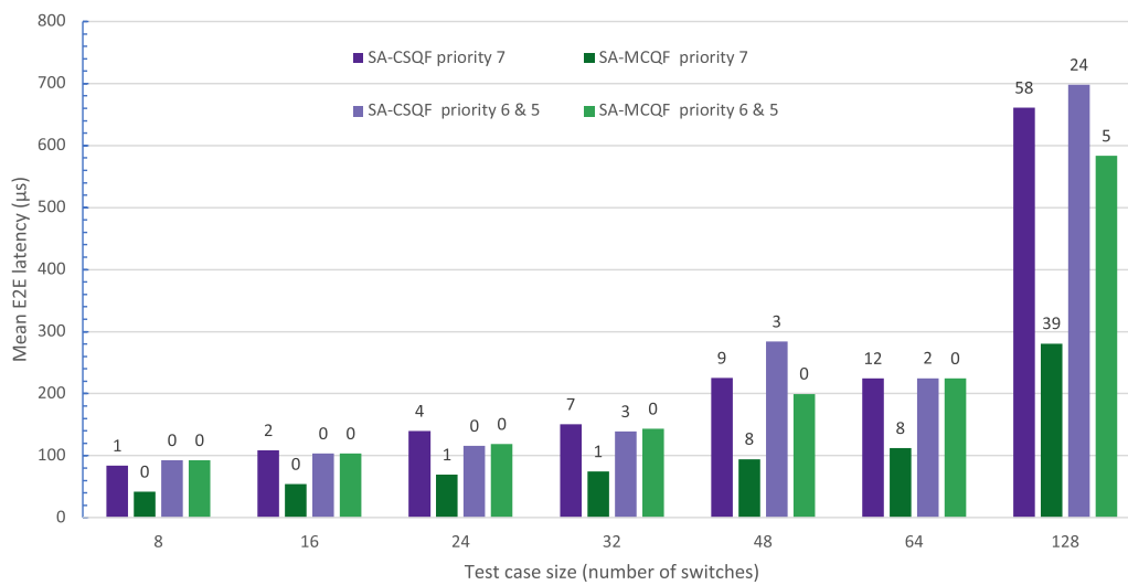
FIGURE 6. Evaluation of Multi-CQF compared to CSQF for ring topologies of increasing size.
