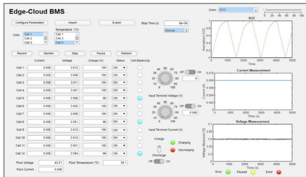
FIGURE 21. Proposed GUI for the BMS access nodes (a) local PC (b) wireless access interface.
