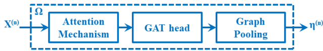
FIGURE 3. GAT block and its components, i.e. the attention mechanism (11), GAT head (12) and graph pooling (13).
