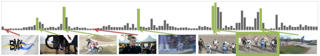
FIGURE 10. Explanation example for a video correctly categorized into class “BMX”. The barplot of frame \beta^{(n)} values (17) is provided at the top of the figure. The two and six video frames with lowest and highest \beta^{(n)} (depicted with red and green bars, respectively) are shown below the barplot. The video frame corresponding to the highest \beta^{(n)} is placed within a green rectangle. We see that the model focuses on the frames that contain at least one bike and ignores other irrelevant ones (e.g. the computer graphics frame, appearing first from the left in the figure). It is also worth noting that the frame selected as the most salient (i.e., with highest \beta^{(n)} ) is the one that depicts multiple BMX vehicles.
