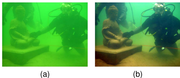
FIGURE 4. Results of the proposed contrast enhancement. (a) Original underwater image (b) Proposed result.
