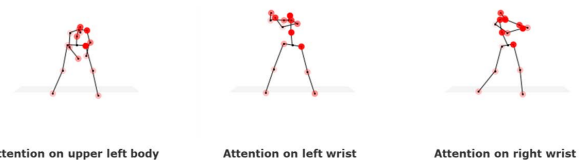
FIGURE 10. Visualization of body parts for revision suggestions. The attention-based network focuses on different body parts at three different phases (address, top, follow-through from left to right). The density and radius of red spheres show the intensity of the attention of the network.
