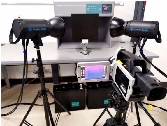
FIGURE 11. The experimental platform of pulsed thermography in Case2.
