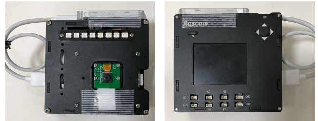
(a) The hardware implementation of our prototype. Our prototype is built based on a camera kit designed for Raspberry pi 4B+ and the Coral USB Accelerator.
