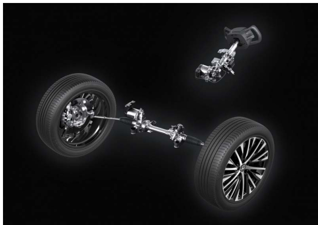
FIGURE 2. Steering system of the Lexus RZ 450e car designed with Steer-by-Wire technology with visible separation of steering column and actuators [2].
