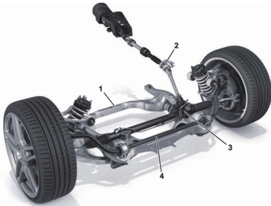
FIGURE 1. Construction of a classic mechanical steering system of the Mercedes-Benz SLS AMG, where the steering column is mechanically connected to the steering rack. 1 – Frame-type integral support, 2- Constant velocity joint, 3 – Steering gear, 4 - Stabilizer bar [6].
