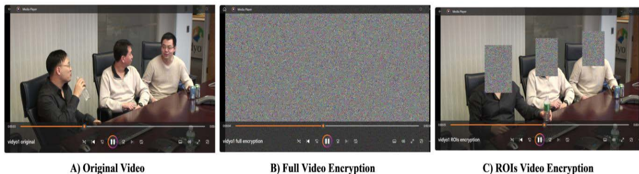
FIGURE 1. Full video encryption and ROIs video encryption.
