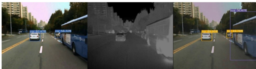
FIGURE 10. YOLOv3 object detection result. VIS image (left); IR image (middle); Fused image (right).
