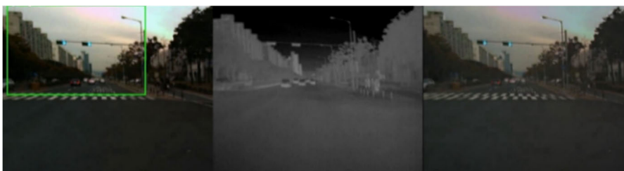
FIGURE 11. SSD object detection result. VIS image (left); IR image (middle); Fused image (right).
