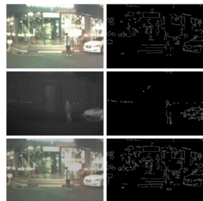
FIGURE 8. Night contour features. Original images (left) and their contours (right); VIS image (top); IR image (middle); Fused image (bottom).
