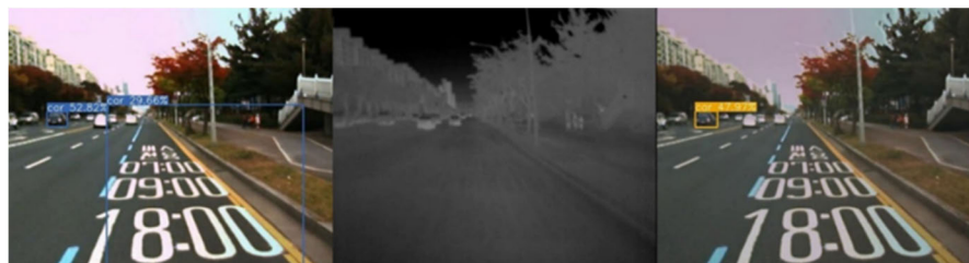
FIGURE 9. YOLOv3 object detection result. VIS image (left); IR image (middle); Fused image (right).
