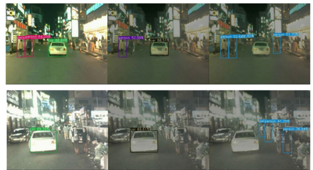
FIGURE 17. Pedestrian detection results in various sample configurations. Training set: VIS image and test set: VIS image (left); Training set: VIS image and test set: fused image (middle); Training set: fused image; test set: fused image (right).
