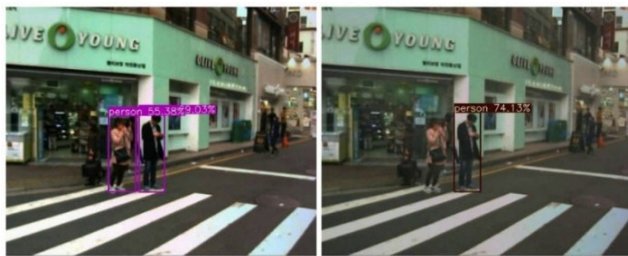
FIGURE 15. Example of performance degradation for the alert objects in daytime. (Left) image before fusion; (right) image after fusion.
