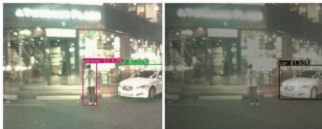
FIGURE 16. Example of performance degradation for the alert objects at night. (Left) image before fusion; (right) image after fusion.
