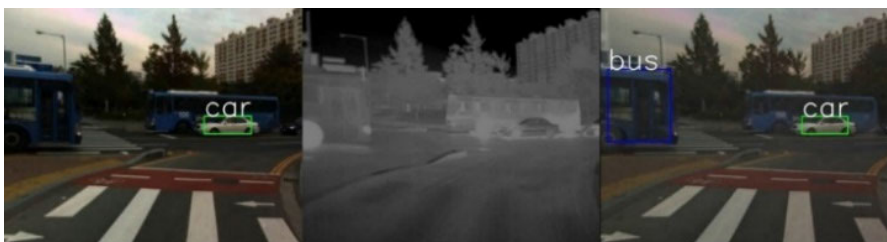
FIGURE 12. SSD object detection result. VIS image (left); IR image (middle); Fused image (right).
