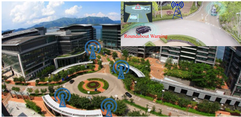
(a) Local-scale roundabout warning of danger ahead using V2X and RSU [144]
