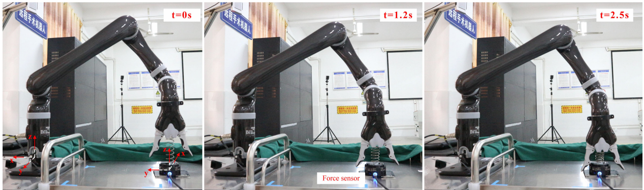
FIGURE 17. Experiment for the elastic force estimation on the end effector.
