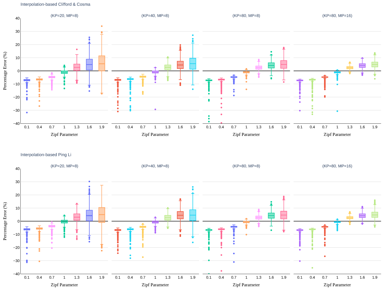
FIGURE 22. Box-and-whisker plot of the relative errors of entropy estimates obtained using interpolation-based LME of Clifford & Cosma (see upper panel) and NECC of Ping Li (see lower panel) schemes for Zipf parameters ranging from 0.1 to 2.0 and different numbers of tables ( kp ) and hash functions ( mp ). The synthetic data stream consists of 300 K items.
