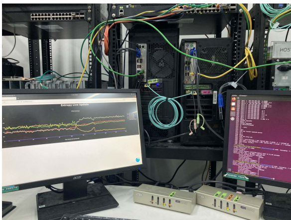
FIGURE 23. FPGA testbed used to evaluate entropy estimation performance with CAIDA 2007 DDoS trace [56].
