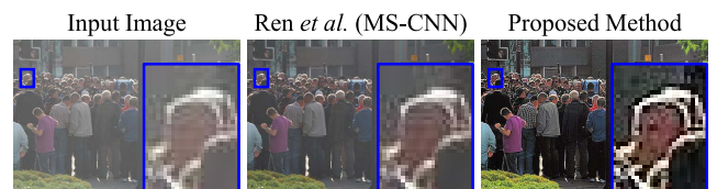
FIGURE 1. A real-world hazy image and its corresponding dehazing results by Ren et al. [3] and the proposed method. MS-CNN stands for the multi-scale convolutional neural network.
