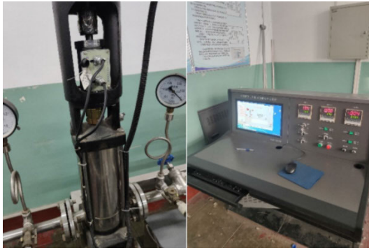
FIGURE 2. Centrifugal pump water supply platform, the various parameters of the centrifugal pump are monitored under this platform.
