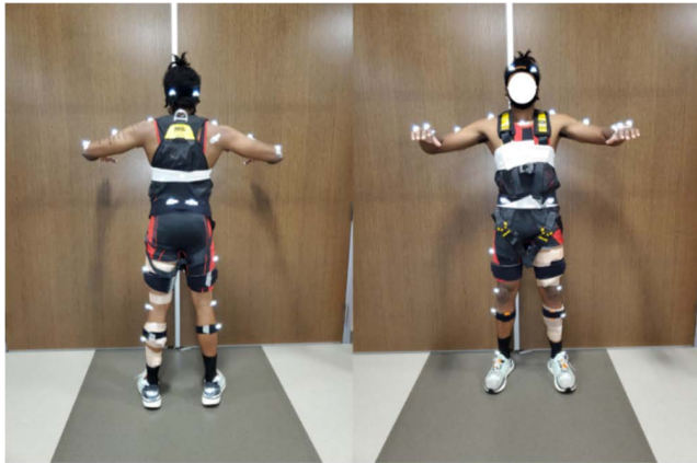
FIGURE 1. Placement of reflective markers and IMU sensors.
