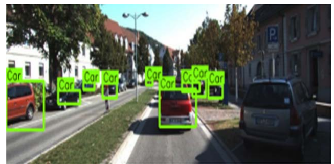
FIGURE 2. Detection of vehicle missed on the right due to presence of a large size, high strength vehicle cast shadow [6].
