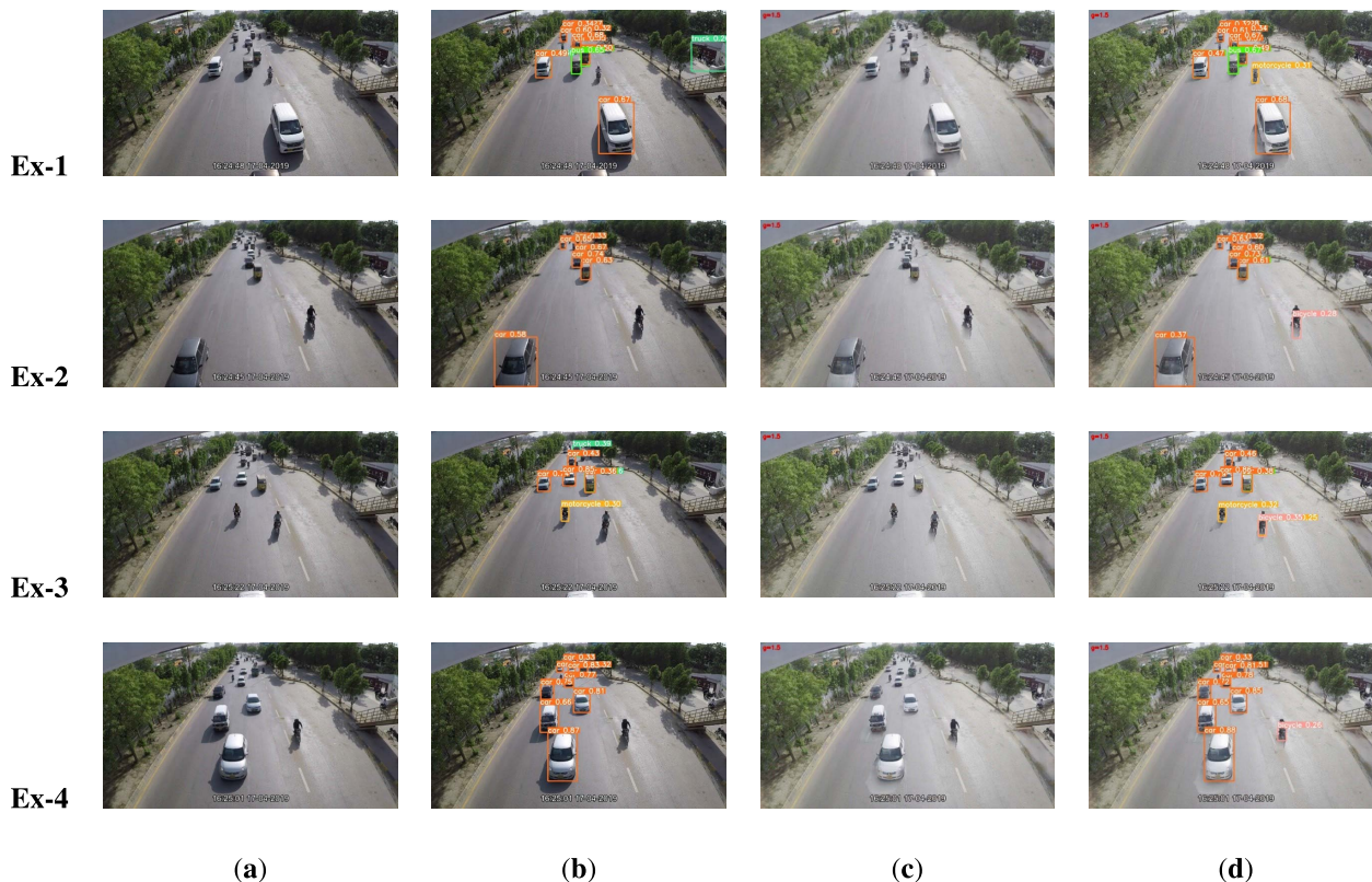
FIGURE 9. Gamma correction and shadow removal, (a) Original image, (b) Prediction (YOLO) on original image, (c) Gamma correction based shadow removal and (d) Prediction (YOLO) after shadow removal.
