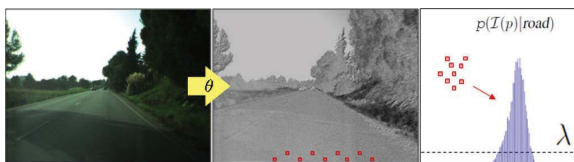
FIGURE 2. Example of using the normalized histogram as a road color model. Figure is from [12].
