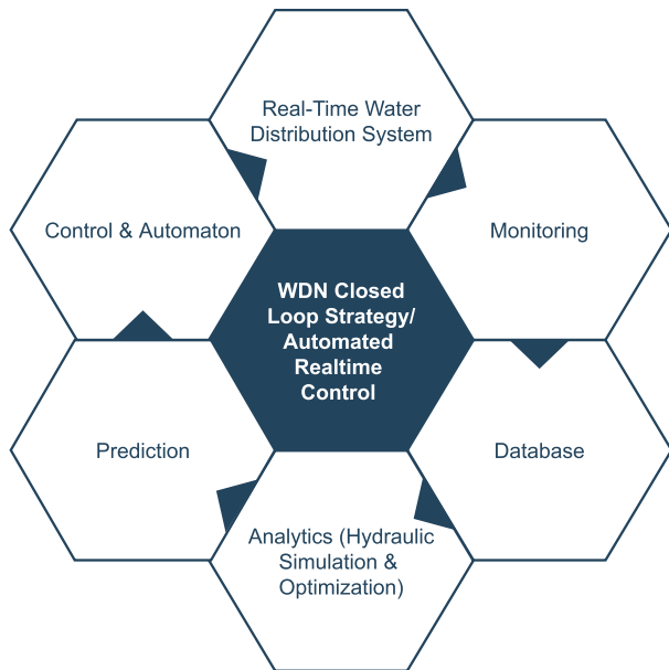
FIGURE 3. Closed-loop strategy for water supply system.
