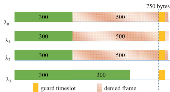
FIGURE 1. The services of an ONU are transmitted on four wavelengths.
