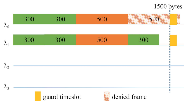
FIGURE 2. The services of an ONU are transmitted on two wavelengths.
