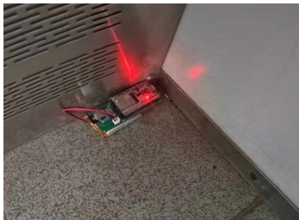
FIGURE 8. The subway vehicle experiment for testing the Intelligent IoT sensing system.
