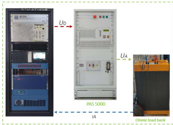
FIGURE 12. Experimental setup of the implemented PHIL simulation system with applied V-ITM interface.
