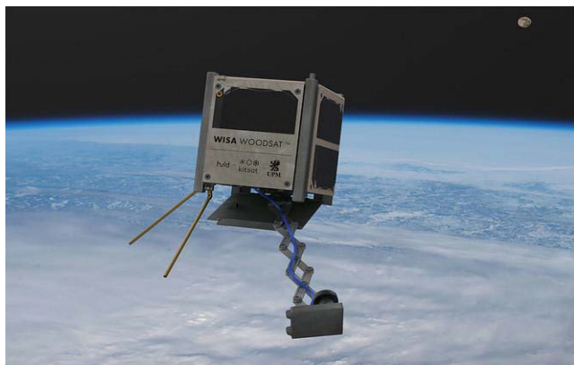
FIGURE 17. WISA WoodSat, a wooden satellite. Credit: Arctic Astronautics.
