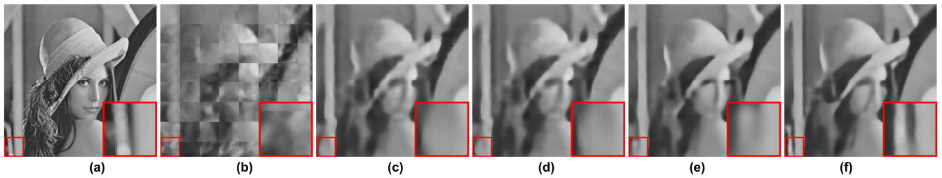
FIGURE 5. Comparison of reconstruction effect on Lena from Set11 with 0.01 sampling rate, (a) Original (PSNR / SSIM). (b) ISTA-Net + (18.54 dB / 0.2557). (c) CSNet + (22.43 dB / 0.6179). (d) SCSNet (22.41 dB / 0.6159). (e) MR-CSGAN (22.84 dB / 0.6446). (f) TDCN (23.33 dB / 0.6646).
