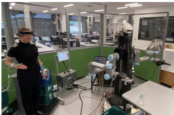
FIGURE 1. Example of a user teleoperating the new dexterity ARoA humanoid robot using an EMG based shared control framework for the execution of complex tasks.
