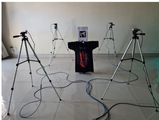
FIGURE 5. Actual view of the sensor setup with a clothing article.
