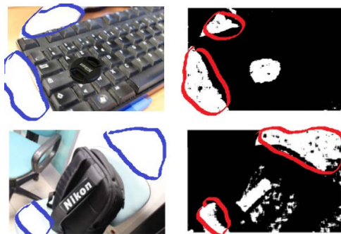
FIGURE 2. An example of falsely detected of PRNU based detector on saturated regions which are limited by blue curves.
