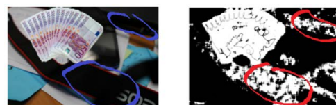
FIGURE 3. An example of falsely detected of PRNU based detector on dark regions which are limited by blue curves.
