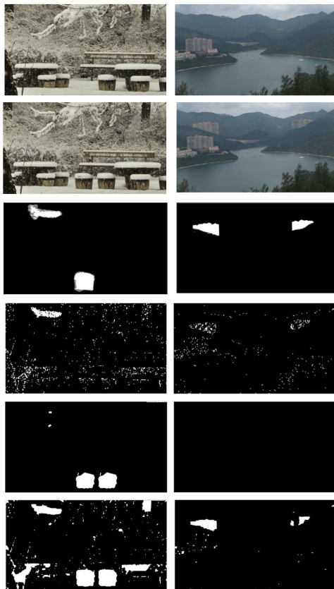
FIGURE 6. Fusion of forensic algorithms improves detection performance by detecting both cut-paste and copy-move forgery regions. These two tampering images are chosen from the dataset of Korus [26]. The first rows are original images, the second row are tampered images, the third row are ground-truth images, the fourth row are maps detected by [62], the fifth row are maps detected by [63] and the last row are integrated maps based on MRF fusion.
