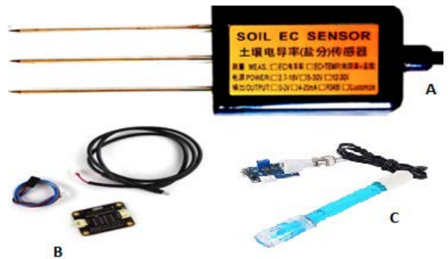
FIGURE 5. Salinity mapping sensors A) MEC-10 Soil EC sensor B) TDS sensor C) pH sensor.
