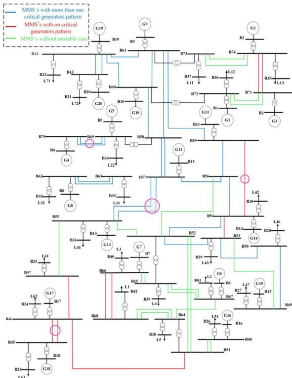
**FIGURE 9.** Single line diagram of the Nordic test system.
