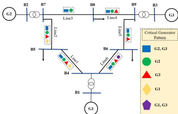
FIGURE 5. Schematic of single line diagram of the IEEE 9-bus system along with critical generator patterns for each line.
