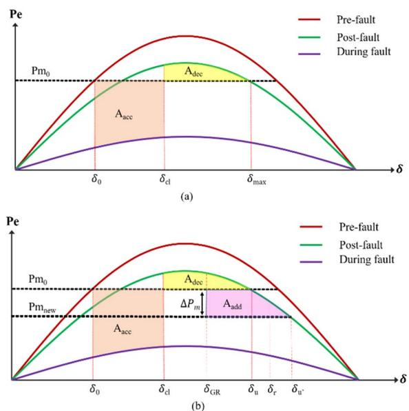
FIGURE 1. Schematic of the EEAC methods to (a) determine the stability status of the power network, (b) determine the amount of required generator rejection to prevent transient instability.
