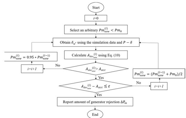
FIGURE 2. Flowchart of generator rejection calculation for an unstable scenario.
