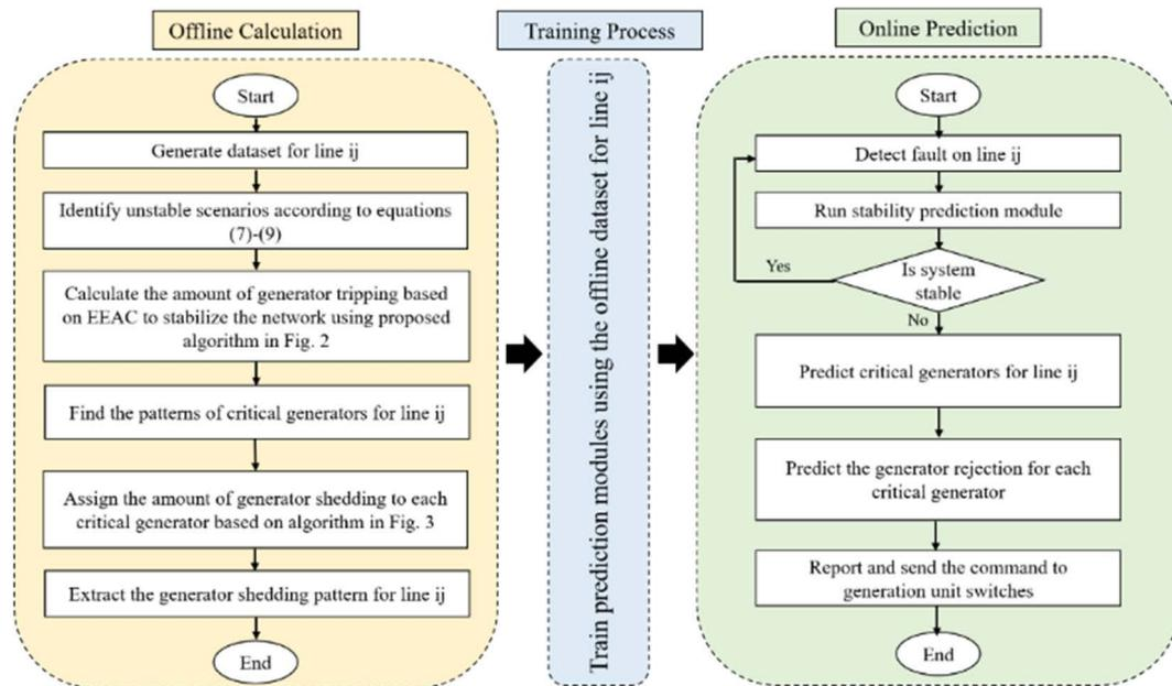
FIGURE 4. A comprehensive diagram of the proposed framework to predict optimal generator rejection for line  $ij$ .
