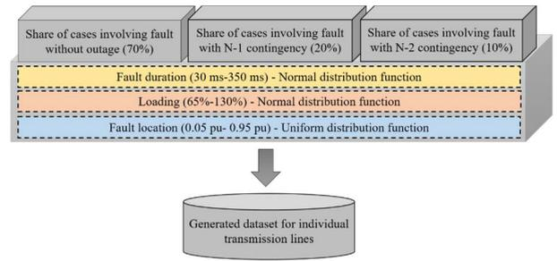
FIGURE 6. Scenario generation process for individual transmission lines.
