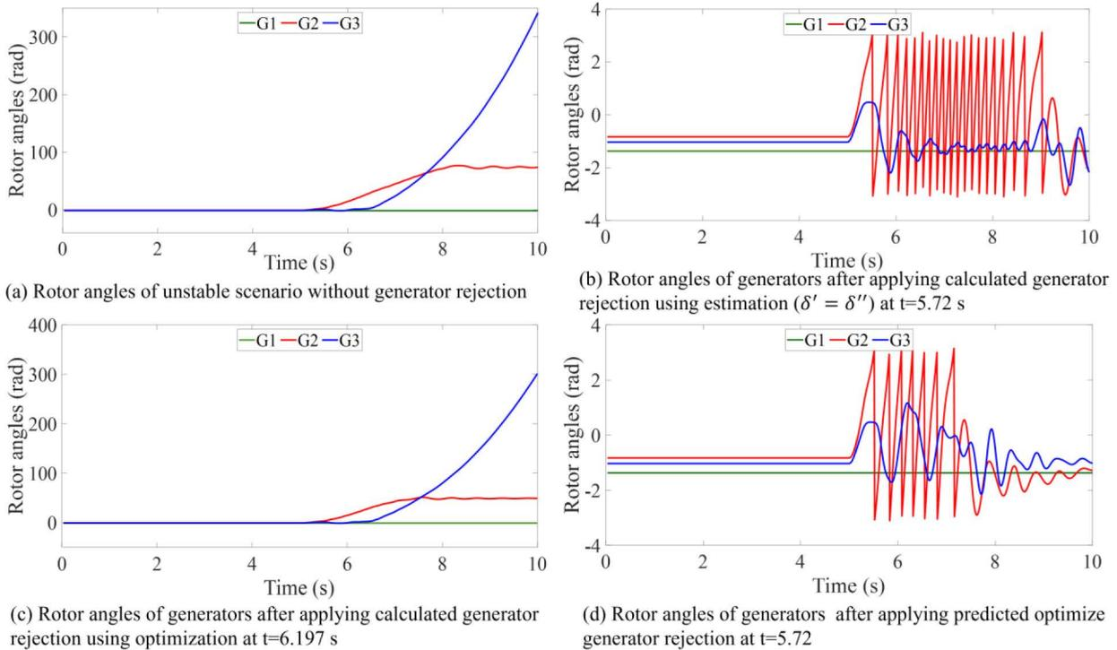
**FIGURE 7.** The rotor angles of generators after applying different generator rejection strategies for a specific case study in the IEEE 9-bus system, (a) the scenario without RCA, (b) scenario after applying RCA based on estimation methods, (c) Scenario after applying optimization-based RCA, (d) Scenario after applying proposed RCA.
