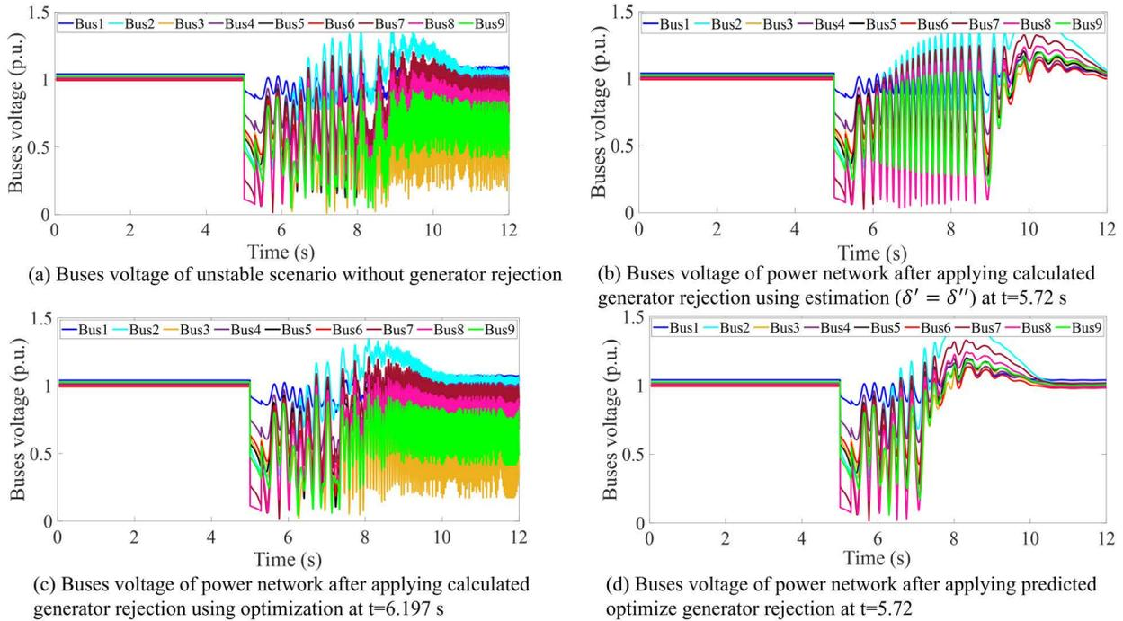
FIGURE 8. Voltage magnitudes after applying different generator rejection strategies for a specific case study in the IEEE 9-bus system.
