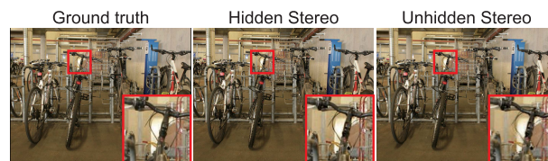
FIGURE 20. Comparison of synthesized images. Ground truth view is shown on the left. Both HS and ES images are generated based on the same per-pixel per-band disparity map. Stereo images generated by the Unhidden Stereo method sometimes exhibit artifacts due to mismatches in high-frequency-band disparity, as seen in the enlarged area. HS can suppress these artifacts by limiting the amount of disparity shift to \pi/4 for each band.
