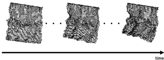
FIGURE 10. Actuator movements can be described as time-series point clouds.
