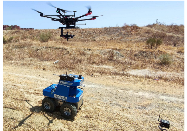
FIGURE 4. UAV and UGV looking for potential victims (position of BLE nodes labeled BE and Aranet).
