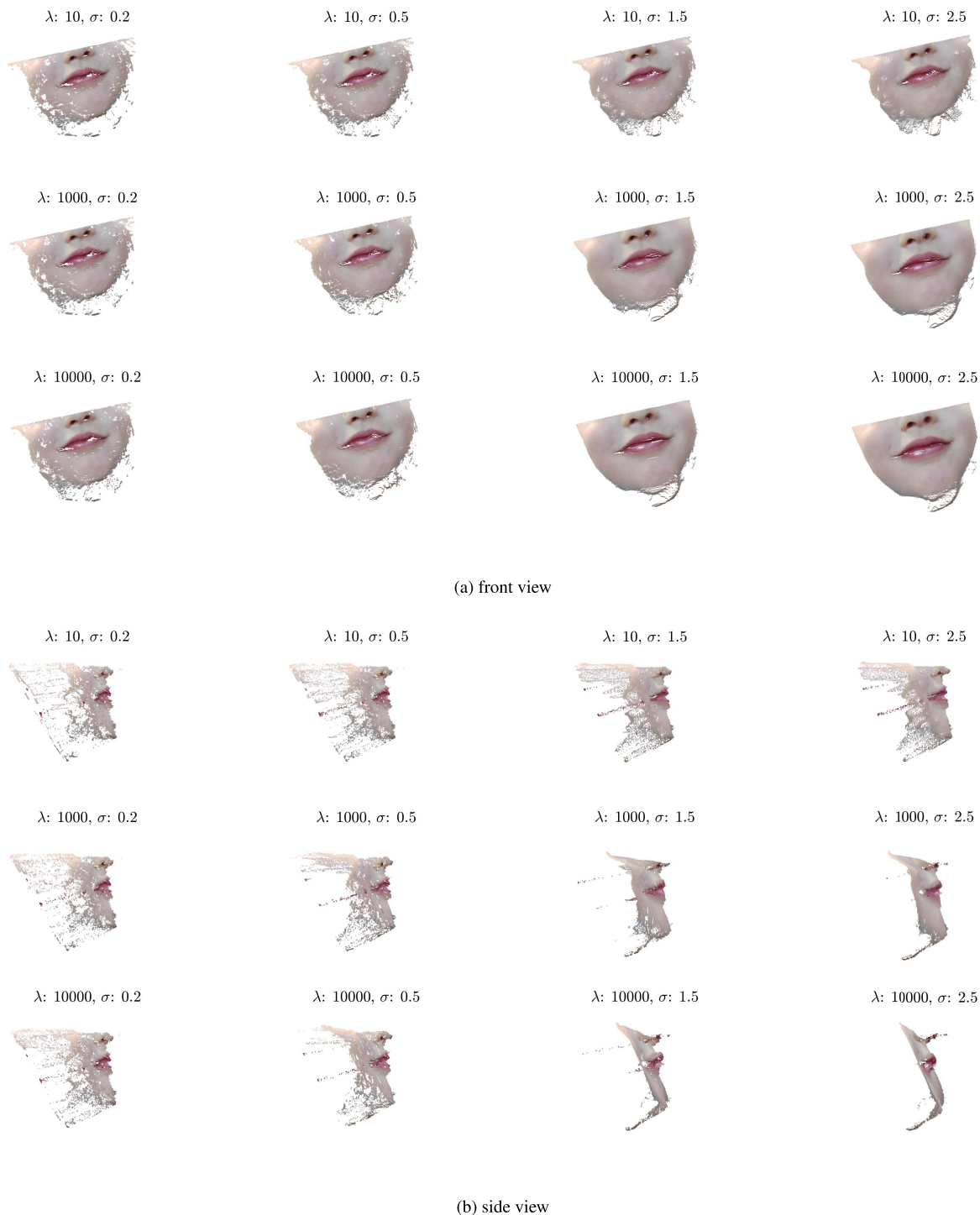
FIGURE 13. Textured point clouds produced from disparity maps by different \sigma (fixed in columns) and \lambda (fixed in rows) in the front (a) and side (b) views.
