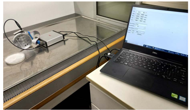
FIGURE 1. Experimental setup of Petri dish with the measured sample and the low-cost electronic nose inside the laminar flow cabinet, connected to the laptop controlling the operation and collecting data.
