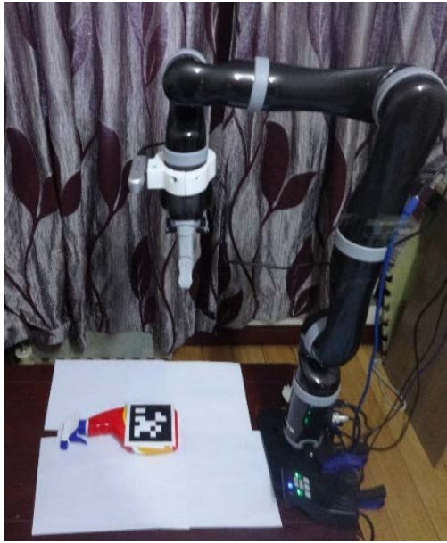
FIGURE 2. Experimental setup: Kinova robotic arm eye in hand configuration with an object carrying an April tag.
