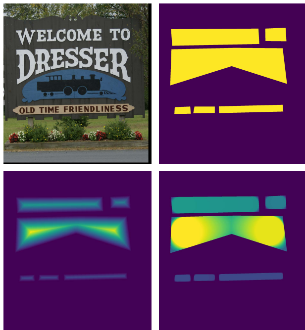
FIGURE 6. Label Generation: The top-left is the original image and its downscaled versions, and on the top-right, their corresponding text instances mask. The bottom-left is the Border distance map, and the bottom-right is the text height map for the input image and its downscaled versions.
