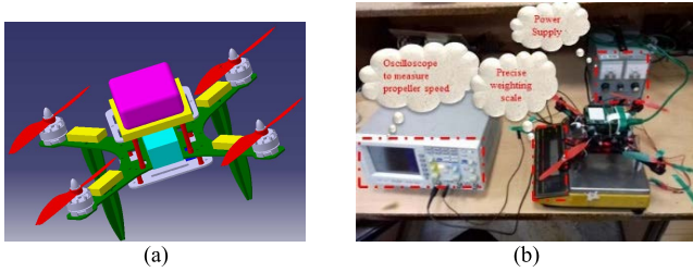
FIGURE 2. (a) Simulated quadrotor with CATIA software, (b) experimental setup to achieve thrust parameter.
