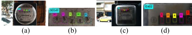
FIGURE 18. Meter reading results. (b) Result of reading a dirty dial meter from (a). (d) Result of reading a dark cyclometer from (a).
