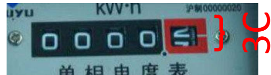
FIGURE 14. The case of an "in-between" digit in a cyclometer.
