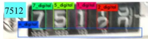
FIGURE 20. Failure case of meter reading due to the problem of “carry-out”. The correct result is “7511”.
