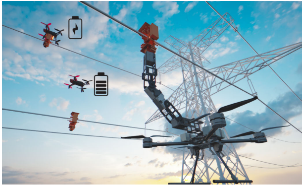
FIGURE 1. Illustration of AERIAL CORE project task to autonomously deploy the recharging station with a drone, an aerial manipulator, and a special robot end effector to increase the autonomy rate of drones power line inspection and monitoring.
