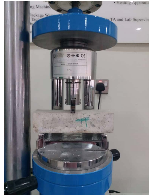
FIGURE 1. Snapshot showing the compression test for one reinforced concrete sample in a controlled laboratory.
