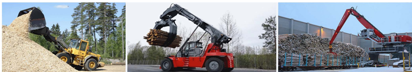
FIGURE 1. Examples of wood handling vehicles: From left to right: Volvo L90E wheel loader shaping a pile of wood chips, RTD3126 TW Log Stacker, manufactured by SKS Toijala Works Oy handling a bundle of industrial roundwood logs, and Mantsinen 300 material handler unloading train wagons.
