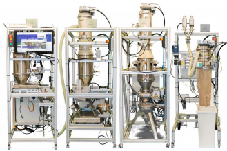
FIGURE 7. BGS. From left to right: loading, storage, weighing, and filling.
