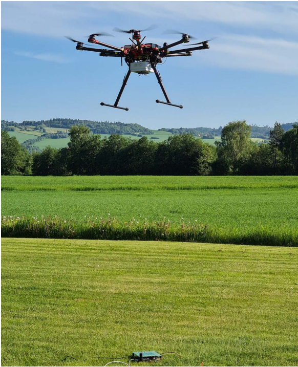
FIGURE 16. Multirotor UAV flying above the array, which is placed flat on the ground facing upwards. The PCB trace antenna on the transmitter board was used.
