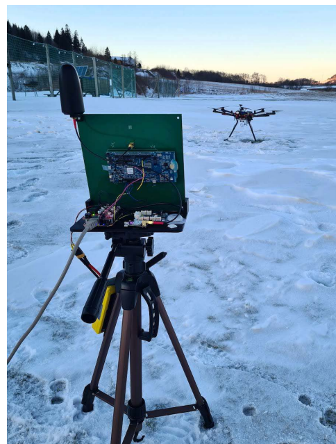
FIGURE 31. The antenna array on a tripod, with array center height 0.7 m over the ground. The DJI S1000 UAV in visible in the background.
