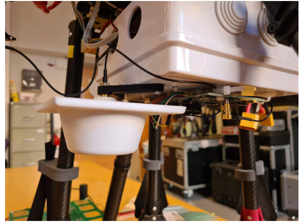
FIGURE 19. RHCP antenna mounted on the multirotor UAV, pointing downwards.
