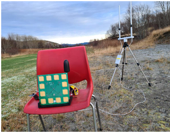
FIGURE 22. Array setup with Ubiquiti Rocket radio for remote equipment placement.
